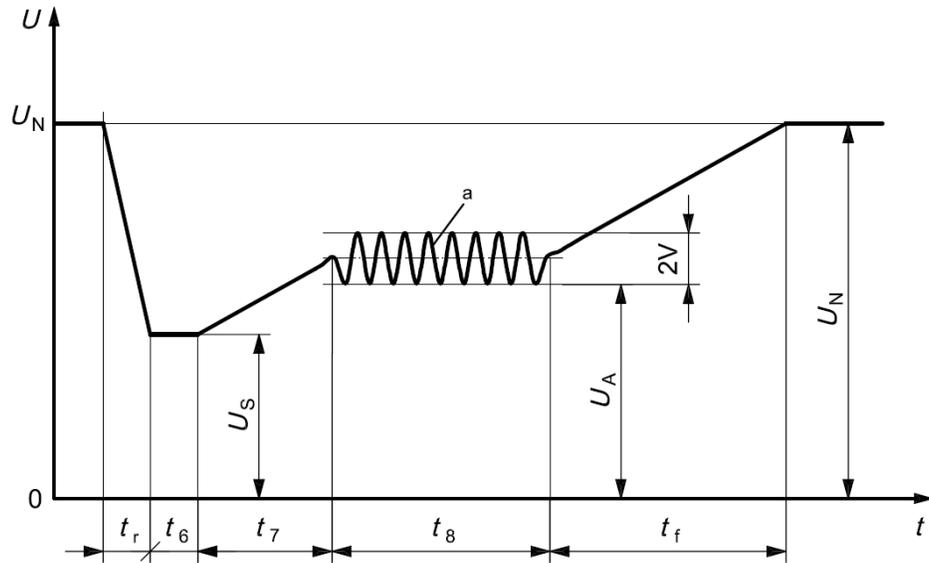
Figure 3.11 – Starting profile waveform
