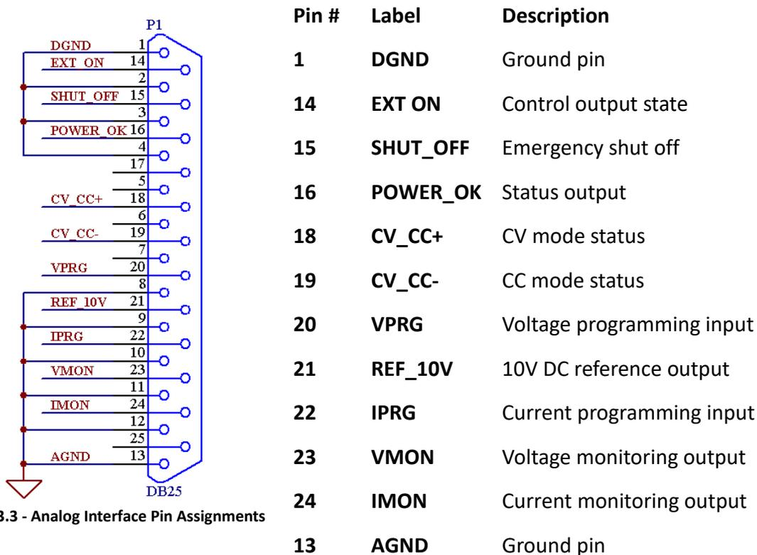
Figure 3.3 - Analog Interface Pin Assignments
