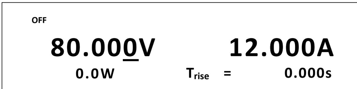
2.  $T_{rise}$  is the rising edge time for an output voltage transition. Use the numeric keypad or the current adjust knob and enter **5.000 s (5 seconds)**.
