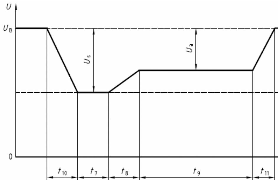
Figure 3.8 – Test Pulse waveform (DIN 40839)
