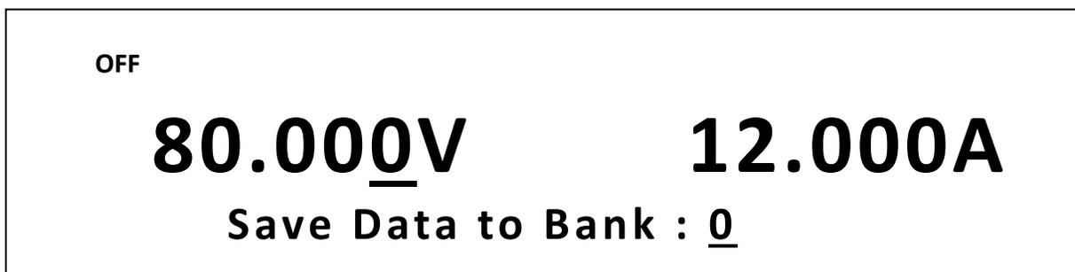
3. Use the current adjust knob or the numeric keypad to enter the memory location in which to store current instrument settings. Select between **0 – 9**. Press
