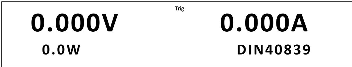
7. To enable the DIN40839 function, press the
