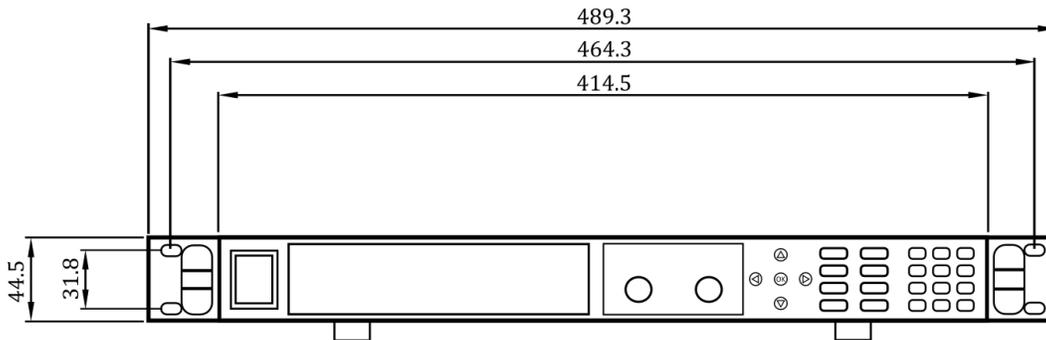
Figure 1.1 - Front Panel View for 9115/B/9115/B-AT/9116/B
