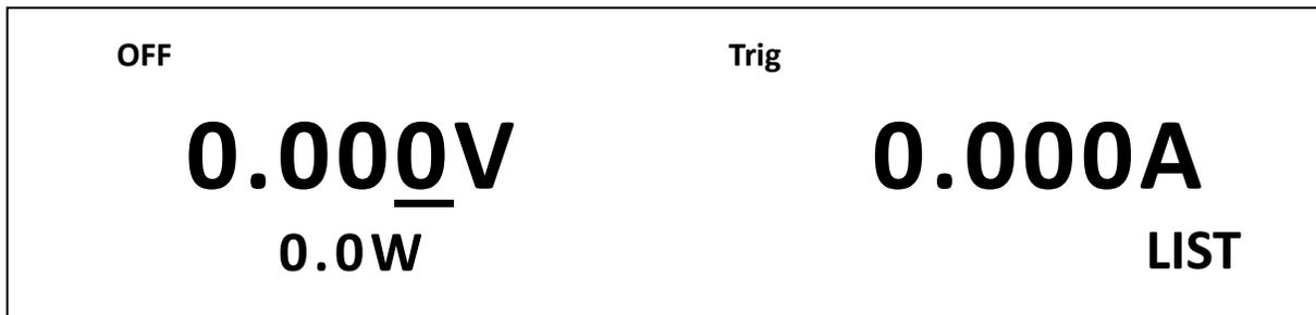
3. If the display is showing the measured voltage and current value, the
