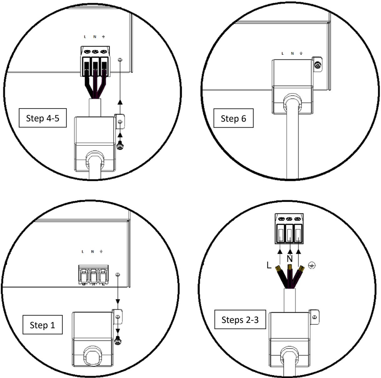
Figure 2.1 – AC Power cable housing assembly
