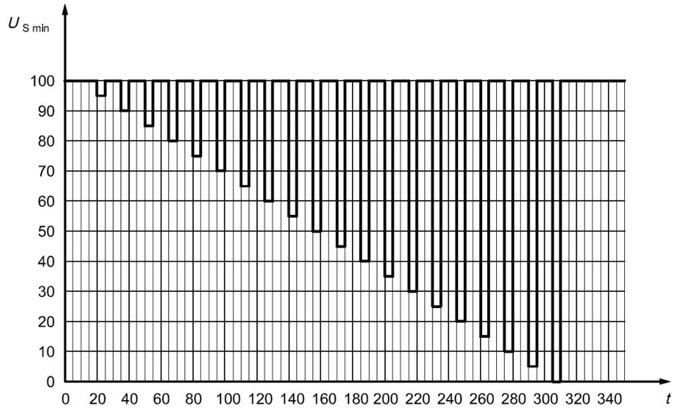
Figure 3.10 – Profile for the reset test waveform
